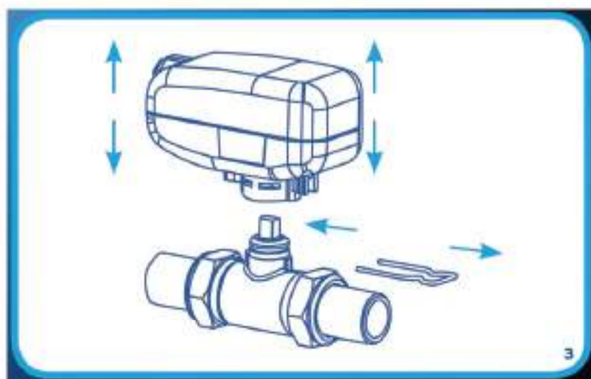
3. THE QUICK connection system allows the servomotor to hook/unhook without disconnecting the valve from the hydraulic circuit.
