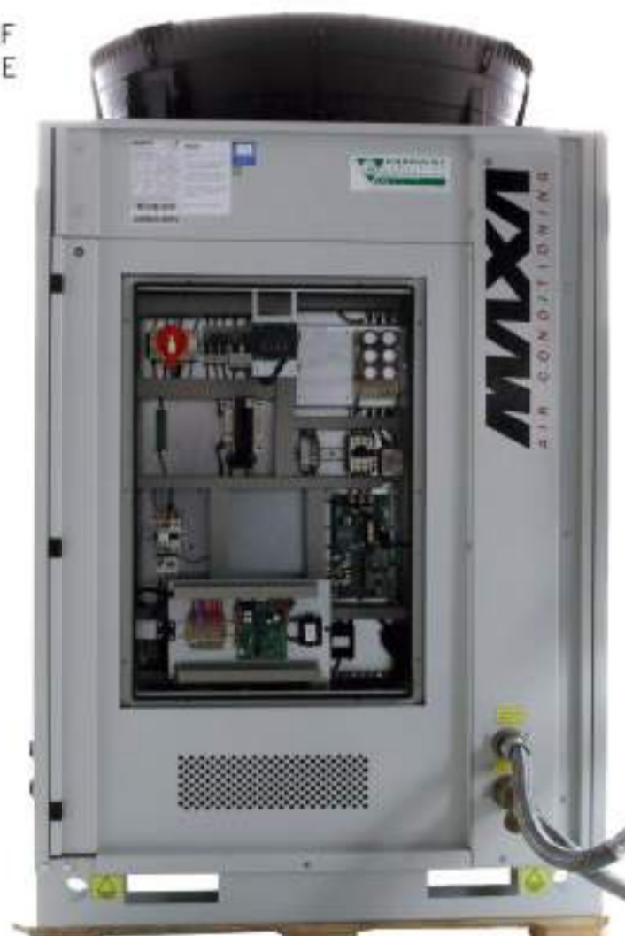
I-HP 250F VERSION. Full inverter with both inverter compressors, with working range between 30 and 80 Hz with frontal view of the electronics on silenced version.
